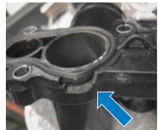
Fig. 3: Breakage (damage pattern)
