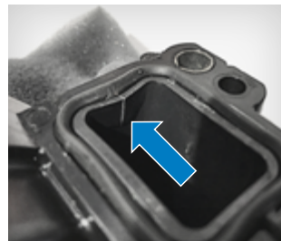
Fig. 2: Breakage (damage pattern)
